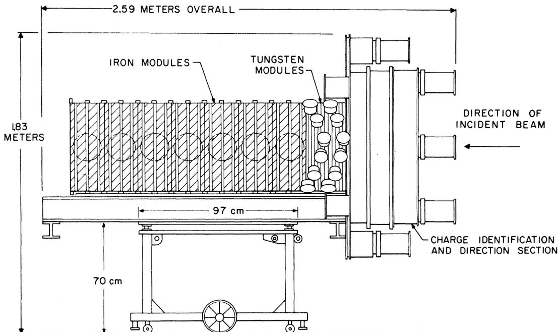
FIG. 1. A schematic view of the high-energy cosmic-ray ionization spectrometer used in this experiment.
