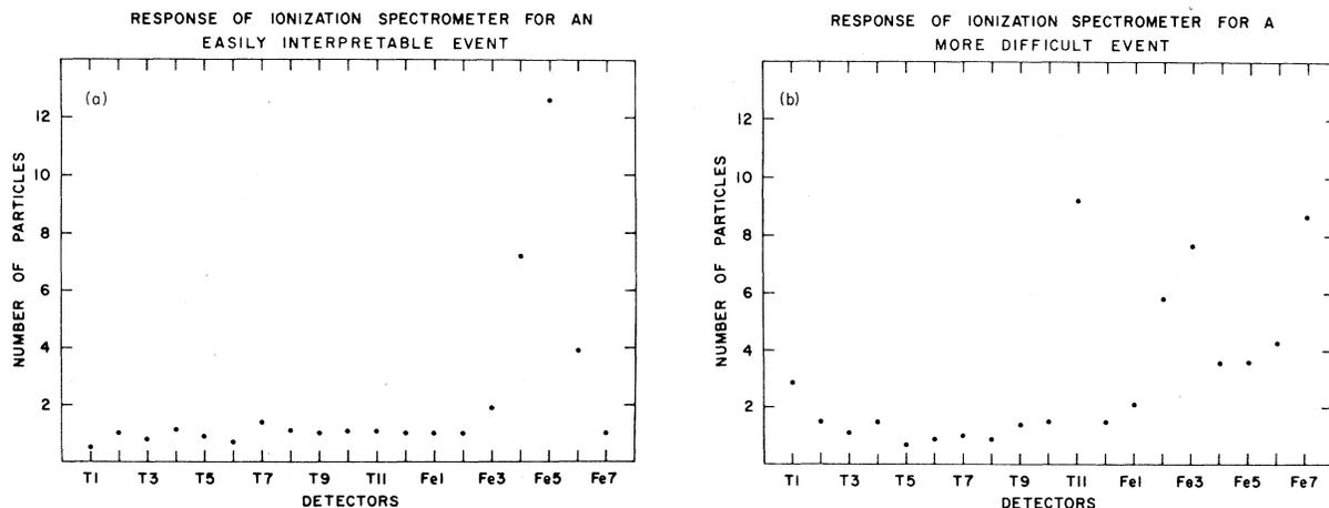
FIG. 2. (a) Plot of pulse height as a function of module number. In this case the module in which the interaction occurred is clearly Fe3. (b) Plot of pulse height as a function of module number. This plot shows the difficulty of making a unique selection of the interaction module.
