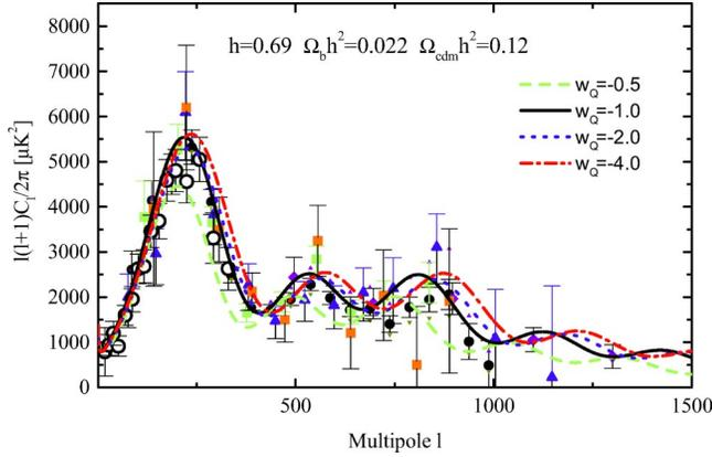
FIG. 1. The effect of varying  $w_Q$  on the Cosmic Background Explorer– (COBE)-normalized CMB angular power spectrum and present CMB data. Since the shift of the power spectrum is proportional to  $\mathcal{R}\ell$ , the discrepancy is more important for higher values of  $\ell$ .
