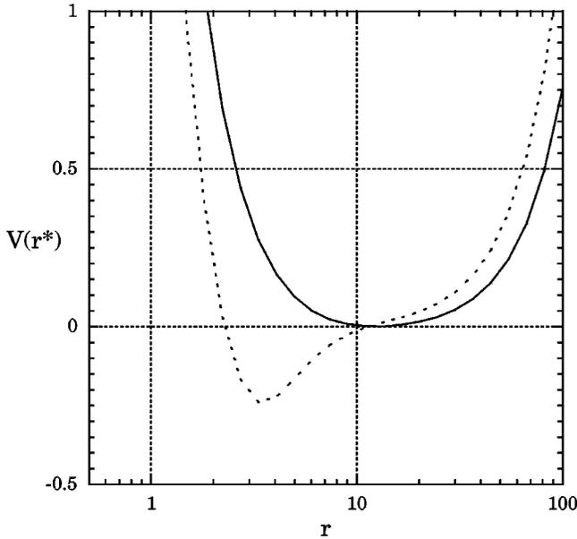
FIG. 17. Potential  $V(r_*)$  for  $\epsilon=1$ . The solid and dotted lines denote those for  $b=-0.01$  and  $b=-0.1$ . There is a negative region [ $V(r_*) < 0$ ] for  $b=-0.1$  but the result is positive definite for  $b=-0.01$ . We set  $\ell=10$ .
