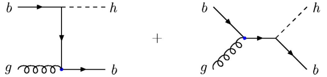
FIG. 3. Diagrams for the next-to-leading-order correction to b\bar{b} \rightarrow h from initial gluons. This correction is of order 1/\ln(m_h/m_b) .
