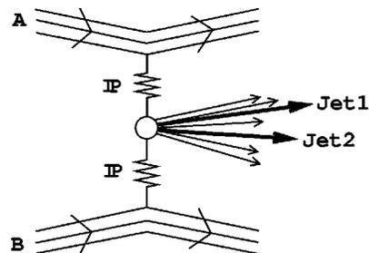
FIG. 1. Schematic view of hadrons  $A$  and  $B$  interacting via double Pomeron exchange and giving rise to dijets in the central region.
