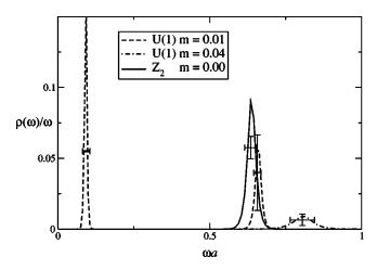
FIG. 13. Rescaled Bryan image of  $\rho(\omega)/\omega$  in the  $\sigma$  channel from time slices 1–10 at  $\beta$ =0.65, for two different masses in the U(1) model on a 32<sup>2</sup>×24 lattice, and for m=0 in the  $Z_2$  model on a 24<sup>3</sup> lattice.
