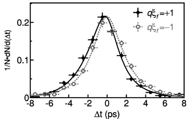
FIG. 2. The  $\Delta t$  distributions for the events with  $q\xi_f = +1$  (solid points) and  $q\xi_f = -1$  (open points). The results of the global fit with  $\sin 2\phi_1 = 0.719$  are shown as solid and dashed curves, respectively.
