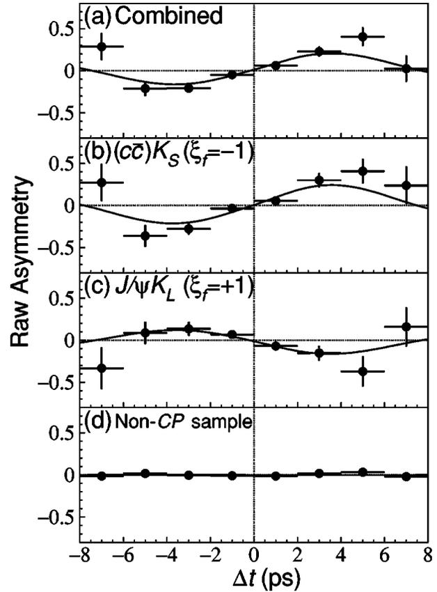
FIG. 3. (a) The raw asymmetry for all modes combined. The asymmetry for  $J/\psi K_L^0$  and  $J/\psi K^{*0}$  is inverted to account for the opposite  $CP$  eigenvalue. The corresponding plots for (b)  $(c\bar{c})K_S^0$ , (c)  $J/\psi K_L^0$ , and (d) non- $CP$  control samples are also shown. The curves are the results of the unbinned maximum likelihood fit applied separately to the individual data samples.
