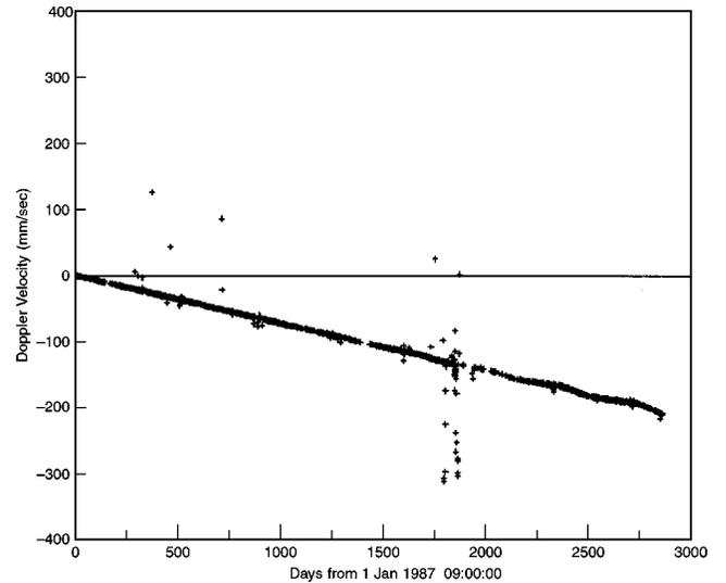
FIG. 8. CHASMP two-way Doppler residuals (observed Doppler velocity minus model Doppler velocity) for Pioneer 10 vs time. 1 Hz is equal to 65 mm/s range change per second. The model is fully relativistic. The solar system’s gravitational field is represented by the Sun and its planetary systems [49].
