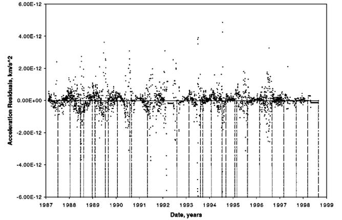
FIG. 17. ODP 1-day batch-sequential acceleration residuals using the entire Pioneer 10 data set. Maneuver times are indicated by the vertical dashed lines.
