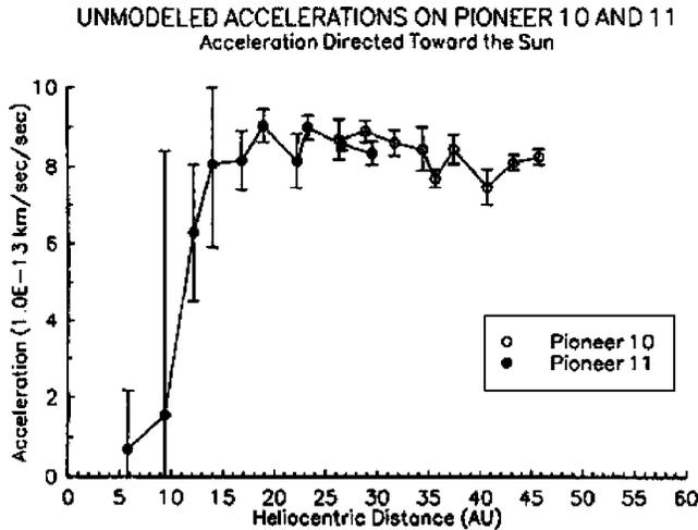
FIG. 7. An ODP plot of the early unmodeled accelerations of Pioneer 10 and Pioneer 11, from about 1981 to 1989 and 1977 to 1989, respectively [75].
