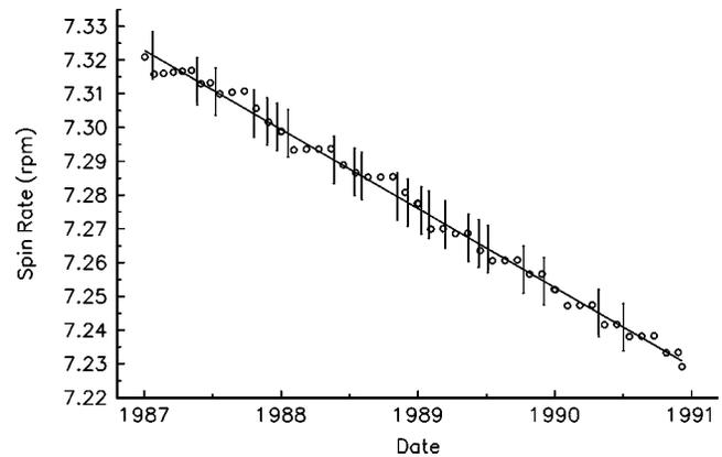
FIG. 12. The spin history of Pioneer 11 over the period of analysis. The vertical lines indicate the times when precession maneuvers were made. This spin calibration was done by the DSN until 17 July 1990. At that time the DSN ceased doing spin calibrations. From 1990 until the loss of coherent Doppler, orbit analysts made estimates of the spin rate.
