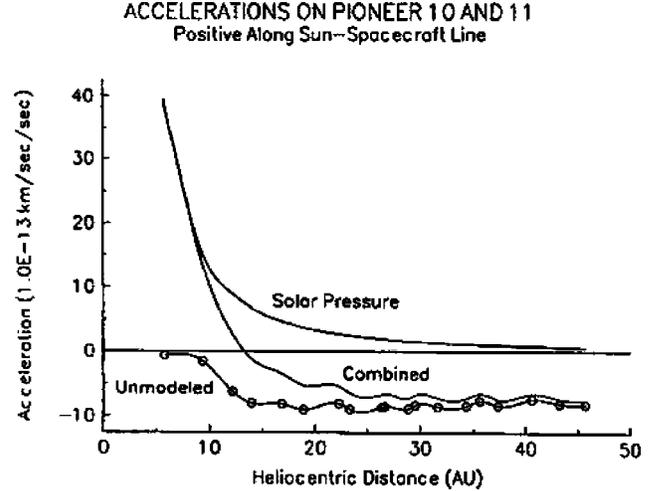
FIG. 6. ODP plots, as a function of distance from the Sun, of accelerations on Pioneers 10/11. The accelerations are (a) the calculated solar radiation acceleration (top line), (b) the unmodeled acceleration (bottom line), and (c) the sum of the two above (middle line) [75].
