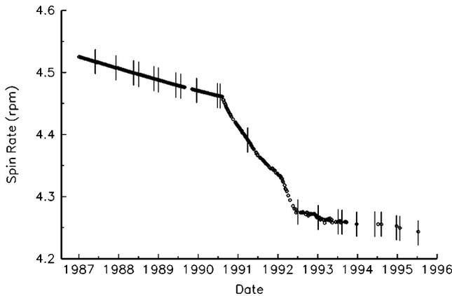
FIG. 11. The spin history of Pioneer 10. The vertical lines indicate the times when precession maneuvers were made. How this spin data was obtained is described in Sec. III E. The final data points were obtained at the times of maneuvers, the last being in 1995.
