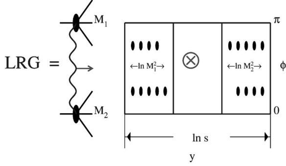
FIG. 1. Lego plot for the double Pomeron Higgs boson production process.
