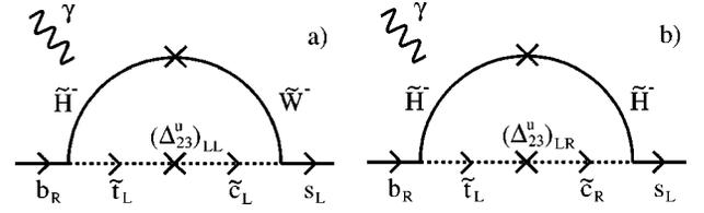
FIG. 33. Diagrams corresponding to the two contributions associated with the chargino amplitude of Eq. (39). In (a) flavor violation is introduced through a  $(\Delta_{23}^u)_{LL}$  mass insertion along the  $\tilde{t}_L - \tilde{c}_L$  squark line. In (b) a  $(\Delta_{23}^u)_{LR}$  mass insertion is introduced along the  $\tilde{t}_L - \tilde{c}_R$  chirality flipping squark line.
