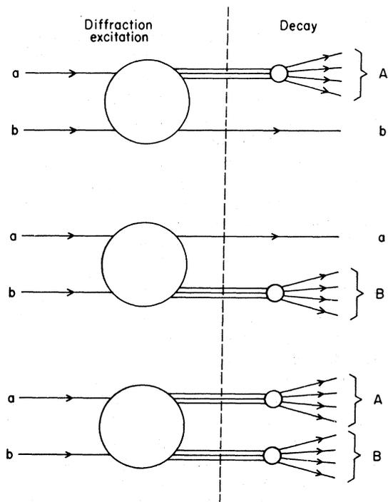
FIG. 3. Graphical representation of diffractive dissociation, in which the incident particle  $a$ ,  $b$ , or both of them are dissociated.
