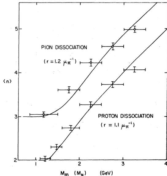
FIG. 4. Average multiplicity of  $X_m$  and  $X_N$  as a function of their invariant mass  $M_m$  and  $M_N$ . The experimental points are from Ref. 3. The curves have been calculated by a statistical model, taking the effective radius of the excited states equal to  $1.2 \mu_\pi^{-1}$  and  $1.1 \mu_\pi^{-1}$ , respectively. See text for the details of calculation.
