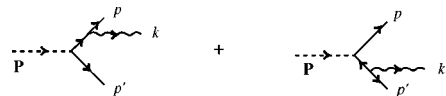
FIG. 1. Diagrams for the radiative corrections to the tree model are shown. A dashed line denotes a meson, a wavy line denotes a photon and a solid line denotes a lepton.
