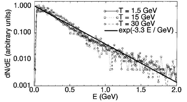
FIG. 17. Linear-log plot of QCD photosphere spectra (normalized to have same peak value) for three different horizon temperatures, and the analytic fit  $dN/dE = \exp(-E/300 \text{ MeV})$ .
