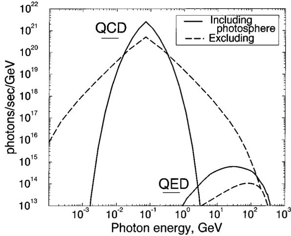
FIG. 19. Photon emission spectrum from  $T=50$  GeV ( $M=2 \times 10^{12}$  g) black hole. Solid lines are spectra which include photospheres. Dashed lines are given for comparison and represent the results for photons from direct quark fragmentation at the horizon and subsequent  $\pi^0$  decay (QCD), and for direct photon emission neglecting the QED photosphere (QED).
