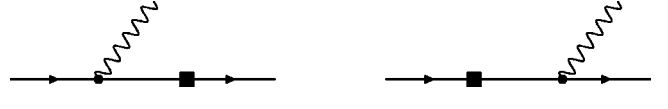
FIG. 1. Diagrams that contribute to radiative hyperon decays. Solid and wavy lines denote ground state baryons and photons, respectively. Solid squares and circles are vertices of the weak and electromagnetic interactions, respectively.
