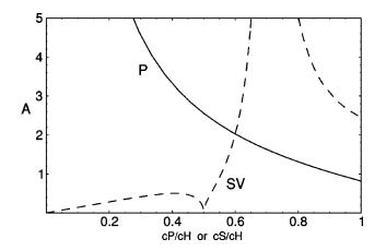
FIG. 3. Anisotropy ratio for waves that propagate upward in a homogeneous half space, reflect off the Earth's surface, and propagate back downward. The curve "P" is for the case when the upward propagating waves are pure P (P-up waves), in which case the abscissa is  $c_P/c_H \equiv \sin \alpha_P$ ; "SV" is for SV-up waves, with abscissa  $c_S/c_H \equiv \sin \alpha_S$ . It is assumed that  $c_P = 2c_S$ ; this is approximately the case for the surface layers at Hanford and Livingston.
