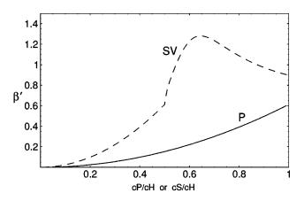
FIG. 4. Reduced transfer function for P-up and SV-up waves in a homogeneous half space with  $c_P = 2c_S$ . Notation is as in Fig. 3.
