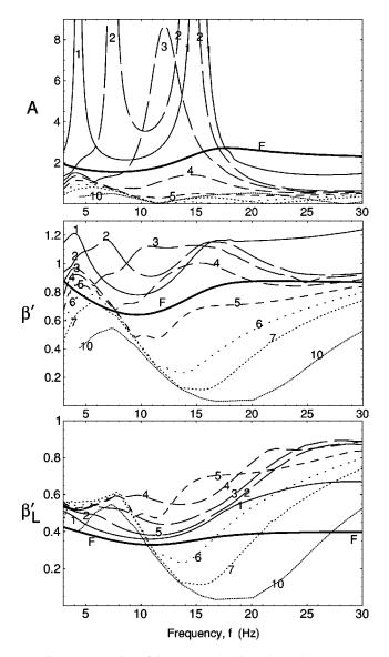
FIG. 10. Properties of the lowest 10 RS modes and the RF mode of the 4-layer Livingston model. (Modes RS8 and RS9 are not shown; their curves are sandwiched between 7 and 10.)
