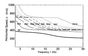
FIG. 9. Dispersion relations for 4-layer Livingston model, including coupling between P- and SV-waves produced at boundaries between layers, for the fundamental mode and the lowest 10 RS modes.
