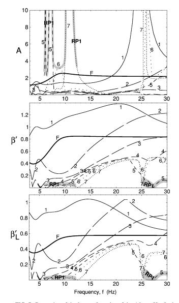
FIG. 7. Properties of the lowest 8 modes of the 4-layer Hanford model, including coupling between P- and SV-waves produced at boundaries between layers and at the Earth's surface.
