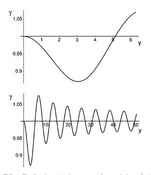
FIG. 1. The function  $\gamma(y)$  that accounts for correlations of seismic gravity-gradient noise in the two corner test masses. This function is given analytically by Eq. (1.19), and it appears in all of the reduced transfer functions:  $\beta_I(f) = \beta'_I(f) \gamma(2\pi f l/c_{HI}) \Gamma_I(f)$ .
