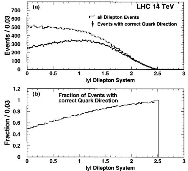
FIG. 1. Rapidity  $|y|$  distribution of the dilepton system with respect to the beam direction for all events and the subsample where the sign of the rapidity agrees with the quark direction (a). The fraction of events with a correctly assigned quark direction is shown in (b).
