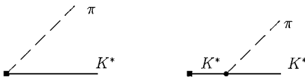
FIG. 2. Feynman diagrams representing the matrix element of the left-handed current from the vacuum to K^* \pi . For the first diagram, the axial vector current contributes while for the second pole diagram, the vector current contributes.
