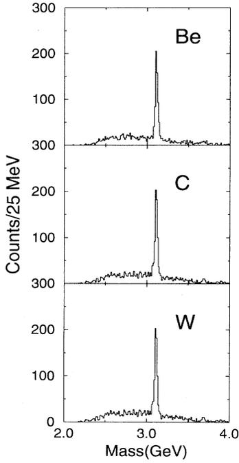
FIG. 1. Dimuon mass spectra for the three nuclear targets integrated over the other kinematic variables (not corrected for acceptance).
