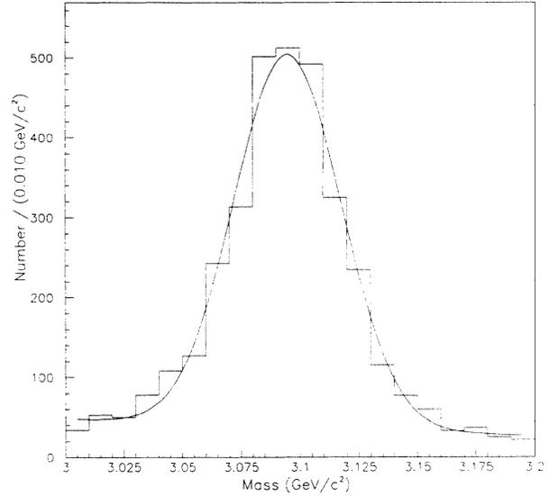
FIG. 2.  $\mu^+\mu^-$  mass distribution after all cuts. The solid curve is a fit to a Gaussian signal plus a linear background giving  $2649 \pm 51 J/\psi$ 's above background.
