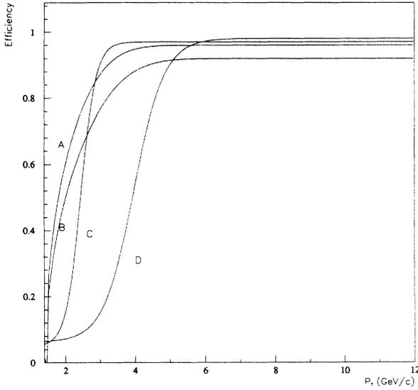
FIG. 1. Muon trigger efficiency parametrizations. Curves A and B show the parametrizations of the 2 and 3 GeV trigger requirements for level 1, respectively. Curves C and D show parametrizations of the 3 and 5 GeV/c charged track requirement for the muon triggers, respectively.
