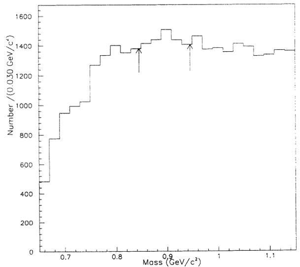
FIG. 3. Invariant mass distribution of track pairs with  $K^\pm\pi^\mp$  mass assignments. Candidate  $K^*(892)^0$  mesons were selected from the region within  $\pm 0.050$  GeV/c<sup>2</sup> of the  $K^*(892)^0$  mass as shown by the location of the arrows.
