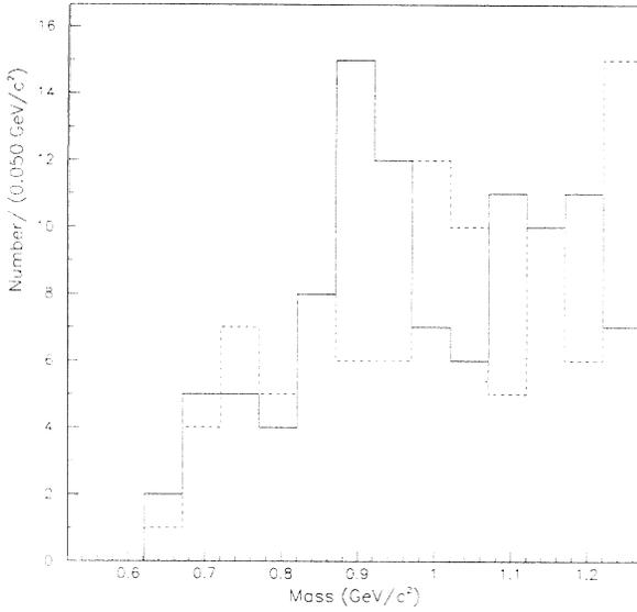
FIG. 6.  $K^*(892)^0$  mass distribution for events in the  $B^0$  mass window (solid line) and for events in the  $B^0$  sideband region (dashed line). Both  $K^+\pi^-$  and  $K^-\pi^+$  combinations are plotted.
