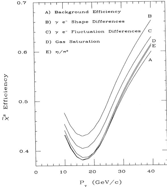
FIG. 22. Simulated background  $\tilde{\chi}^2$  efficiencies. Also shown are the  $1\sigma$  upper systematic uncertainties due to shower fluctuations, shower shape, gas saturation, and the  $\eta/\pi^0$  ratio.
