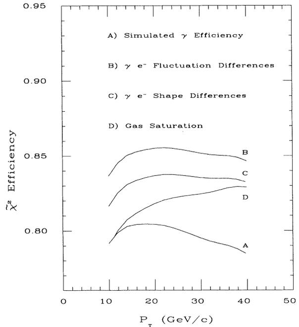
FIG. 21. Simulated photon  $\tilde{\chi}^2 < 4 / \tilde{\chi}^2 < 20$  efficiencies. Also shown are the  $1 \sigma$  upper systematic uncertainties due to shower fluctuations, shower shape, and gas saturation.
