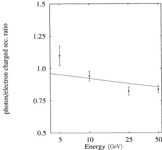
FIG. 11. The number of electrons plus positrons impinging on the chamber sensitive volume for photon showers divided by the number for electron showers versus energy. The curve is from the parametrization used in the simulation. The data points are from a simulation using GEANT.
