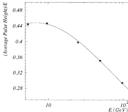
FIG. 10. The average pulse height observed in the strip chamber divided by the beam energy. The data points are for test beam electrons and the solid line is the parametrization used in the simulation.
