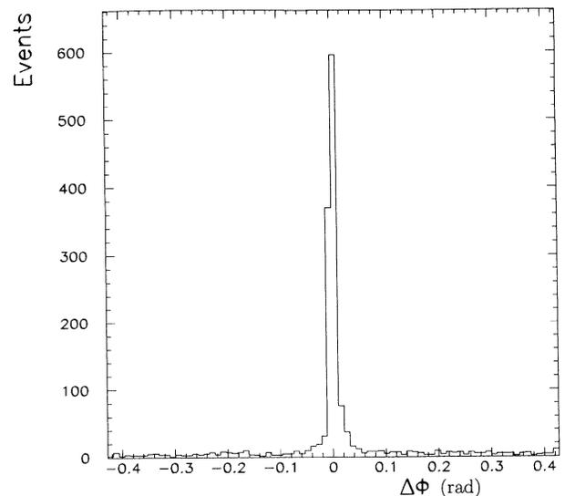
FIG. 24. The difference between the  $\phi$  observed in the CTC compared to the value observed in the CDT for tracks that satisfy a tight cut in  $|\Delta z|$ .
