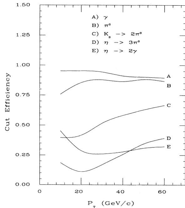
FIG. 16. The fraction of simulated particles passing the CDF selection criteria.
