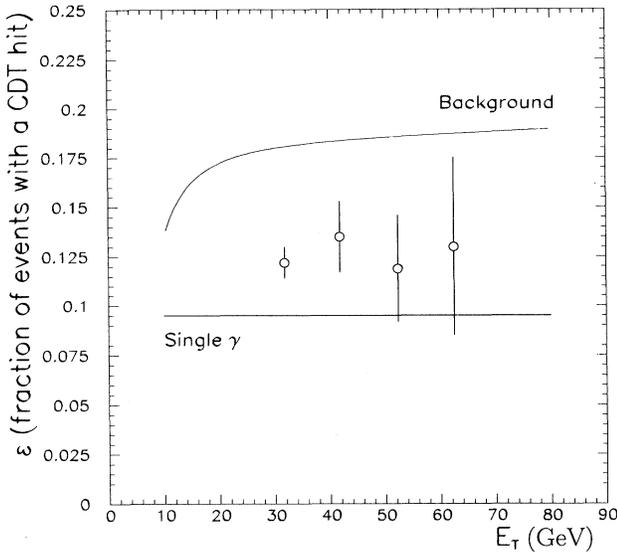
FIG. 29. The expected CDT hit rate for background and single  $\gamma$  events (solid lines). The data points are the observed hit rate with error bars indicating the systematic uncertainty.
