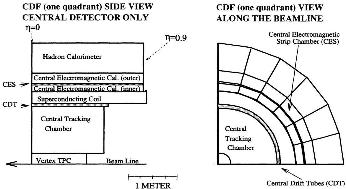
FIG. 2. Cross-sectional view of one quadrant of the CDF central detector.
