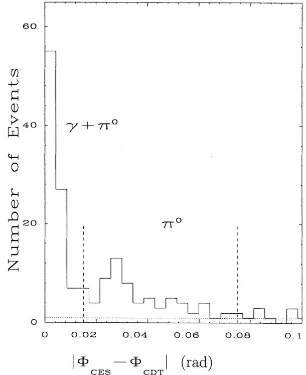
FIG. 27. Difference in azimuth position of the strip chamber cluster and the CDT cluster for 9–11 GeV  $P_T$  photon candidates after a  $\tilde{\chi}^2 < 4$  cut. The  $\tilde{\chi}^2$  cut selects asymmetric decays of the  $\pi^0$ , which are seen as an excess near 0.028 radians.
