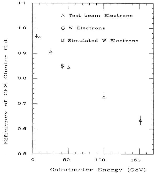
FIG. 7. The efficiency of the second CES cluster cut for different electron energies. The test beam electrons, and electrons from  $W$  decay (both measured and simulated) are shown.
