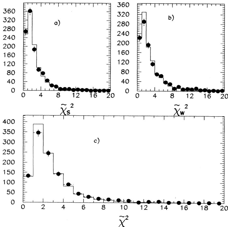
FIG. 12. Comparison of electron  $\tilde{\chi}^2$  from  $W$  decays (points) with a radiative  $W$  Monte Carlo plus detector simulation (histogram): (a) strip view ( $\tilde{\chi}_S^2$ ), (b) wire view ( $\tilde{\chi}_W^2$ ), (c) average of both views ( $\tilde{\chi}^2$ ).
