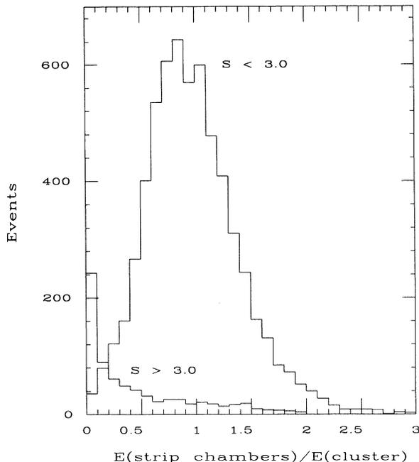
FIG. 8. The strip chamber fractional energy response,  $E(\text{strip chambers})/E(\text{cluster})$ , for two different cases: (1) missing transverse energy significance ( $S > 3.0$ ) signifying a cosmic-ray candidate and (2)  $S < 3.0$  signifying a prompt photon candidate.
