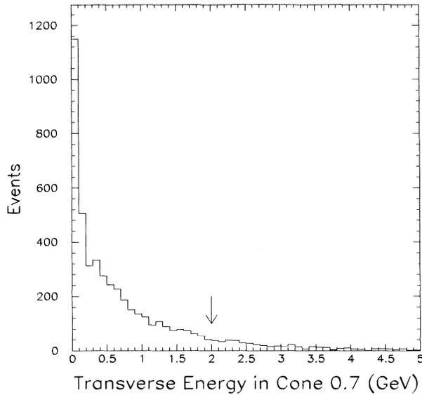
FIG. 6. Transverse energy ( $E_T$ ) in a randomly placed cone of radius 0.7 in a minimum bias event, representing the approximate underlying  $E_T$  expected for direct photon events. The arrow displays the 2 GeV cut value.
