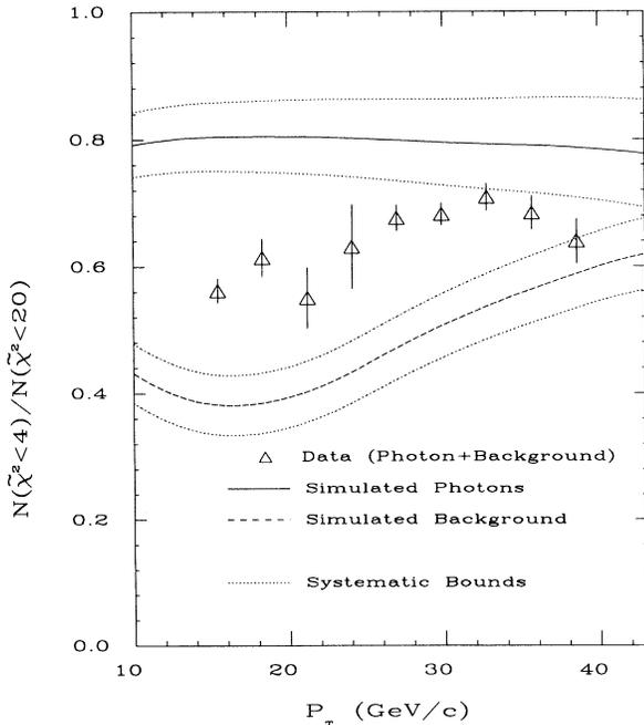
FIG. 23. Signal and background  $\tilde{\chi}^2$  efficiencies for the profile method. Also shown are the total systematic uncertainties on these efficiencies, and the measured efficiency of the data as a function of photon  $P_T$ .
