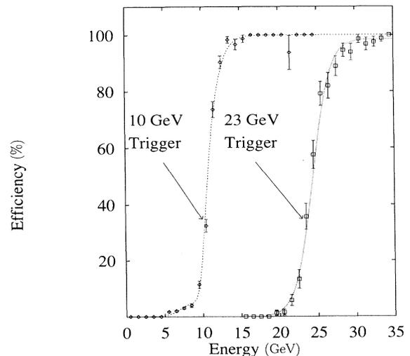
FIG. 5. Trigger efficiencies for the 10 and 23 GeV photon triggers.
