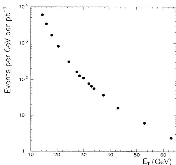
FIG. 9. The  $P_T$  spectrum of the photon candidate events, after all event selection cuts.
