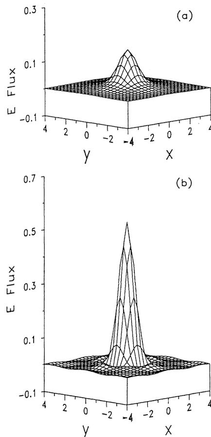
FIG. 1. Surface plot of the electric flux through the  $xy$  plane midway between the  $q\bar{q}$  pair when the system is in (a) the deconfined phase ( $\beta = 1.1$ ) and (b) the confined phase ( $\beta = 0.95$ ). The line joining the pair is located at  $(0,0)$ .
