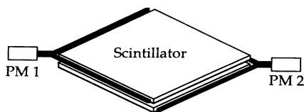
FIG. 6. Construction of a scintillator station, showing the two scintillator plates with the readout by wavelength shifter bars on two sides.
