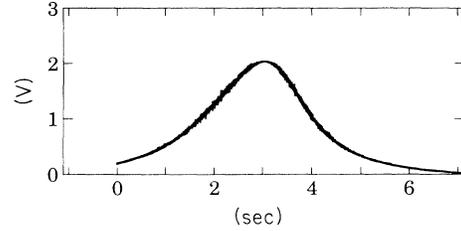
FIG. 6. Noise measurement: dc component of the transmitted intensity. The full width at half height corresponds to  $3.8 \times 10^{-12}$  m. The conversion factor is 0.98 MHz/s or  $1.7 \times 10^{-12}$  m/s.
