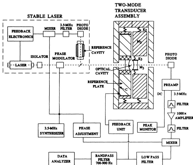
FIG. 1. Layout for the optical transducer.
