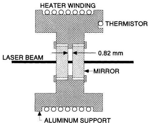
FIG. 2. “Rigid” high-finesse cavity with temperature control.
