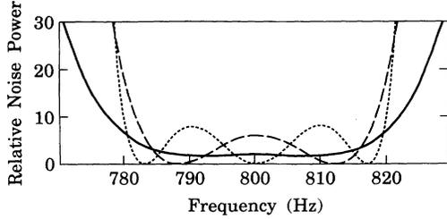
FIG. 9. Thermal noise from the antenna and resonators (solid line), laser back action (long dash), and shot noise (short dash). Unity corresponds to a noise force density of  $4.16 \times 10^{-31} \text{ N}^2/\text{Hz}$ .
