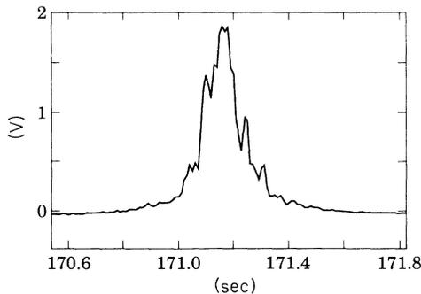
FIG. 5. Finesse measurement: expanded region of the data shown in Fig. 4 showing the fundamental  $i=j=0$  mode of the cavity. The full width at half height corresponds to  $3.8 \times 10^{-12}$  m. The conversion factor is 19.5 MHz/s or  $3.4 \times 10^{-11}$  m/s.
