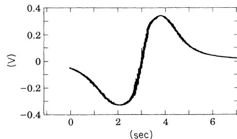
FIG. 7. Noise measurement: rf component of the transmitted intensity. The conversion factor is 0.98 MHz/s or  $1.7 \times 10^{-12}$  m/s.
