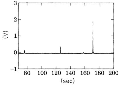
FIG. 4. Finesse measurement: transmitted intensity as the optical cavity expands after heater power offset. The conversion factor is 19.5 MHz/s or  $3.4 \times 10^{-11}$  m/s.
