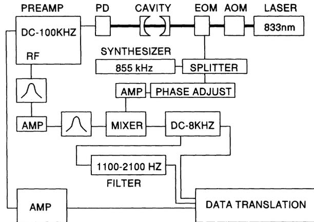
FIG. 3. Electronic layout for the high-finesse cavity.
