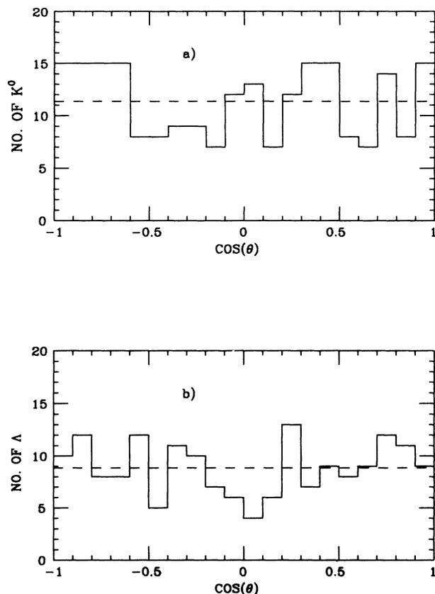
FIG. 1. Distribution of the cosine of the angle between the  $V^0$  line of flight and the negative decay product in the  $V^0$  rest frame, for (a)  $K_S$  and (b)  $\Lambda$ . The dashed line indicates the average number of events in each bin. The distributions are expected to be isotropic.
