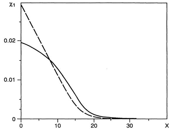
FIG. 3. The dimensionless Bethe-Salpeter wave function  $\chi_1(x)$ , defined in Eq. (4.10), for the exact solution (solid curve) and for the first approximation discussed in Sec. V C (dashed curve). The second approximation was found to be the same as the exact result within the accuracy of the figure. The curves correspond to the model  $G(k^2)=G_1(k^2)$ , Eq. (5.2a).
