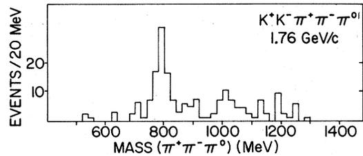
FIG. 4. The three-pion mass spectrum of reaction (4) at 1.76-GeV/c incident momentum.
