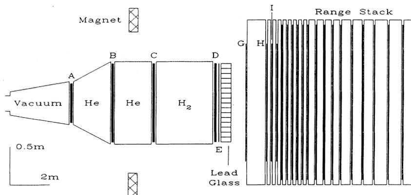
FIG. 1. Plan view of the detector.
