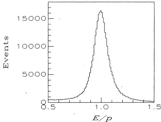
FIG. 4. Distribution of energy deposited in lead glass divided by momentum for electrons from  $K_{e3}$  events.
