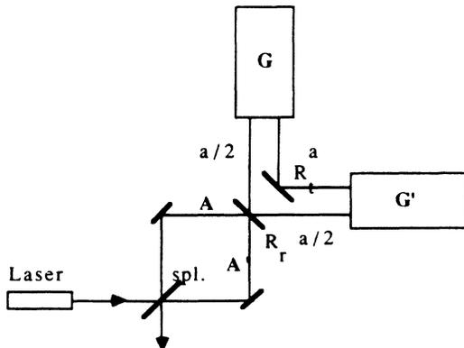
FIG. 9. Sketch of the whole synchronous recycling setup.
