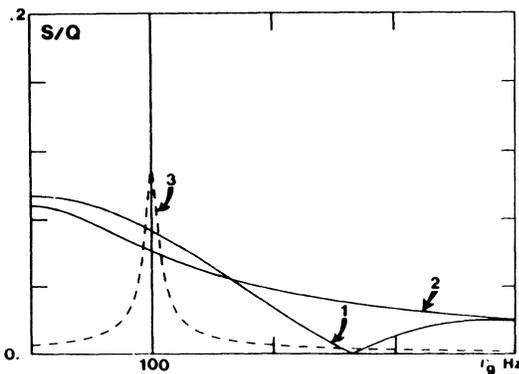
FIG. 6. Transfer function of a Michelson interferometer with multipass arms and standard recycling (optimized at 100 Hz): (1) delay lines; (2) resonant FP cavities; (3) detuned FP cavities.
