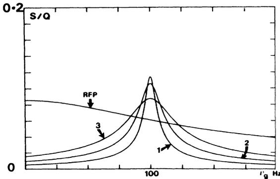
FIG. 7. Transfer function for standard recycling with detuned FP cavities and nonoptimal time constant. (1)  $t = t_{opt}$ ; (2)  $t = t_{opt}/2$ ; (3)  $t = t_{opt}/4$ . RFP: standard recycling interferometer with resonant FP cavities (for comparison).
