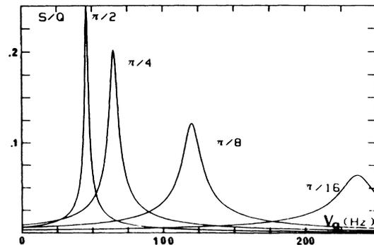
FIG. 13. Transfer functions of a synchronous recycling interferometer with FP cavities at various reflectivity phase ( $\text{Arg}F = \pi/2, \pi/4, \pi/8, \pi/16$ ): tunability.
