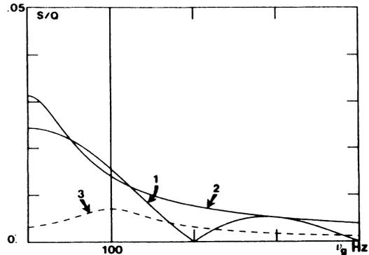
FIG. 4. Transfer function of a Michelson interferometer with multipass arms (optimized at 100 Hz): (1) delay lines; (2) resonant FP cavities; (3) detuned FP cavities.
