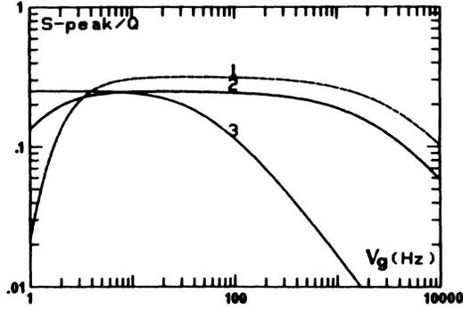
FIG. 14. Synchronous recycling interferometers: peak value of the NSNR: (1) case of delay line; (2) case of FP cavities; (3) standard recycling with detuned FP and optimal time constant (for comparison).
