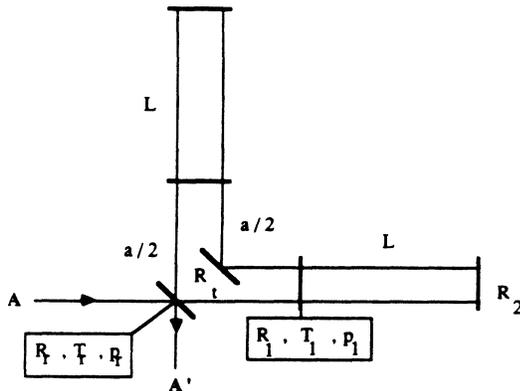
FIG. 12. Synchronous recycling with FP cavities: notation.
