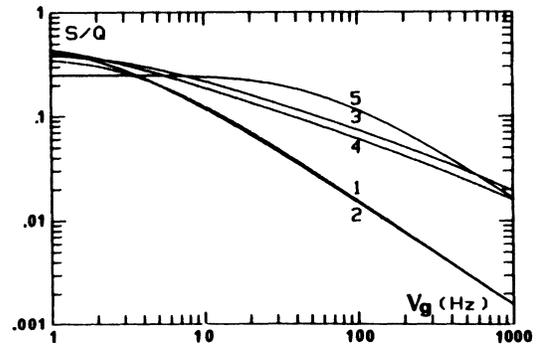
FIG. 8. Optimal values of the NSNR versus gravitational frequency for standard recycling systems: (1) delay lines—no recycling (for comparison); (2) resonant FP—no recycling (for comparison); (3) delay lines—standard recycling; (4) resonant FP—standard recycling; (5) detuned FP—standard recycling (peak value).
