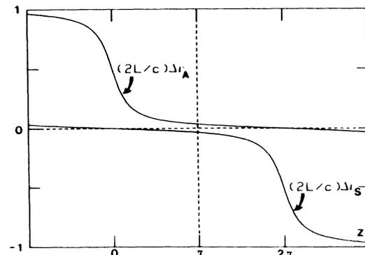
FIG. 11. Eigenfrequencies of a system of coupled cavities.
