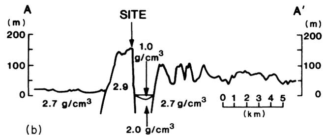
FIG. 3. Geologic and cross-sectional maps of the Palisades site [(a) and (b)]. The line (A-A') labels the trace of the cross section in the geologic maps for the Palisades site. Note the exaggerated vertical scale of the cross section relative to the horizontal scale. Taken from Ref. 13; see footnote 13 therein.
