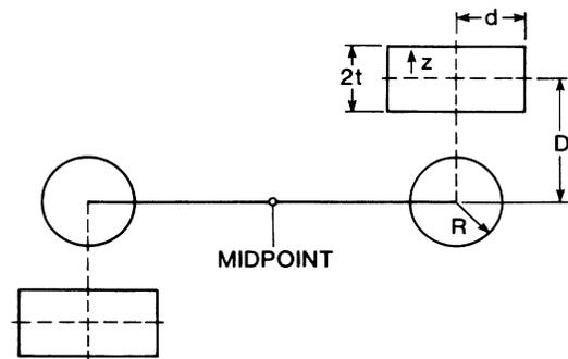
FIG. 5. The geometry of the rotating-disk Cavendish experiment. The spheres have radii  $R$ . Each disk has cylindrical radius  $d$ , thickness  $2t$ , and midpoint a distance  $D$  away from the center of the sphere. The axial coordinate of the disk is  $z$ .
