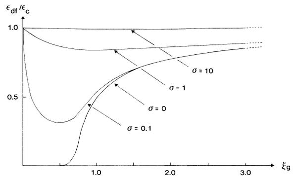
FIG. 1. The energy-density  $\epsilon_{df}$ , defined in the text, normalized to the energy-density  $\epsilon_c$  without the color-singlet condition, for  $x = n_F/N_c = 0.1$  and for various values of  $\sigma = B/N_c$ . ( $B$  is the baryon number.) For  $\sigma = 0$  there is a third-order phase transition at  $\xi_g \approx 0.833$ .
