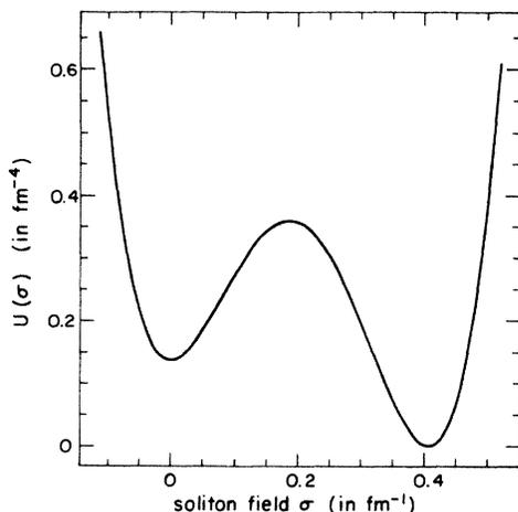
FIG. 1. The soliton field self-interacting potential  $U(\sigma)$  for the following parameters:  $a=51.6$ ,  $b=-799.9$ , and  $c=4000$ .
