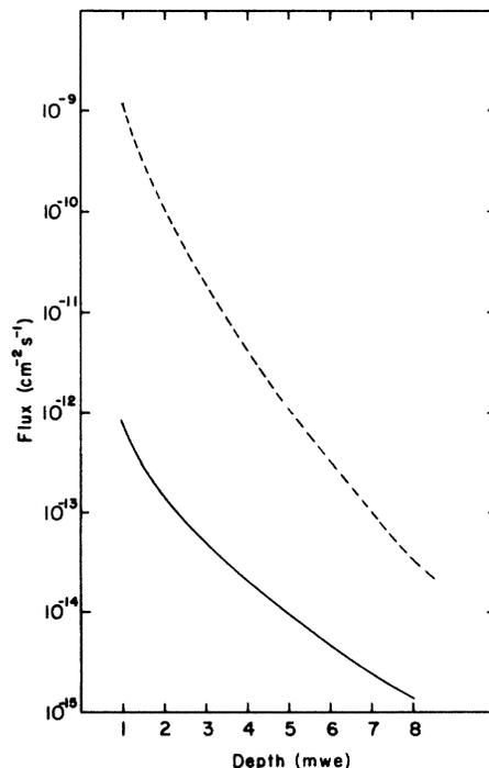
FIG. 4. Vertical flux of  $\gamma$ -induced muons as function of the depth compared to the cosmic-ray muon flux reported in Ref. 16.
