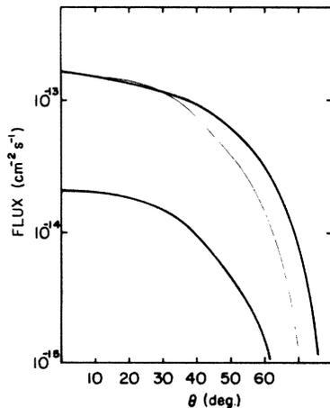
FIG. 3. Angular distribution of muons from  $\gamma$  showers at depths of 2 (upper thick line) and 4 km we. The thin line shows the angular distribution of muons from cosmic-ray hadron showers, normalized to the 2-km we  $\gamma$ -ray line at  $0^\circ$ .
