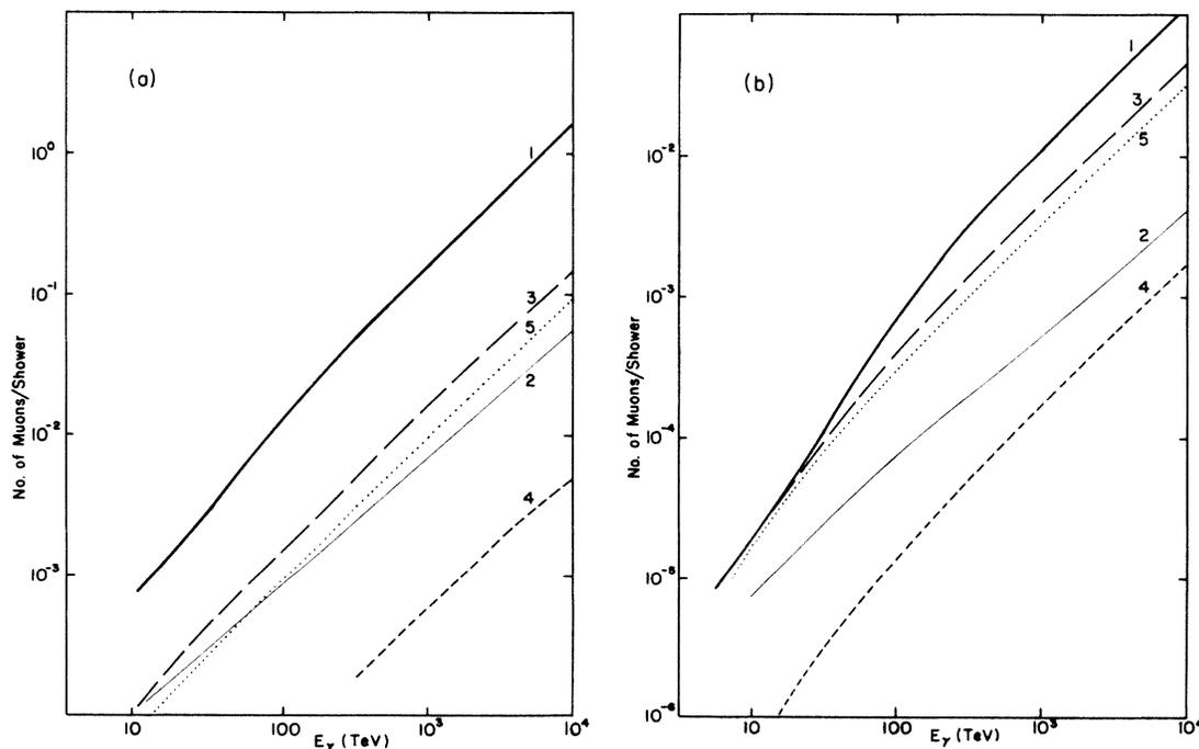
FIG. 2. Muon yields for (a)  $E_\mu > 0.5$  TeV and (b)  $E_\mu > 2$  TeV. Photoproduction: (1) hadrons, (2) diffractive  $\rho$ , (3) charm, (4) bottom. Line (5) shows the QED production of  $\mu^+ \mu^-$  pairs.
