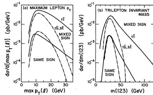
FIG. 5. Distributions of top trileptons with  $p_T > 5$  GeV and opposite-sign pair masses  $> 4$  GeV at  $\sqrt{s} = 620$  GeV; (a) cross sections vs maximum lepton  $p_T$ ; (b) cross sections vs trilepton invariant mass. The contributions from  $t\bar{t}$  (solid curves) and  $t\bar{b}$ ,  $b\bar{t}$  (dashed-dotted curves) are shown separately.
