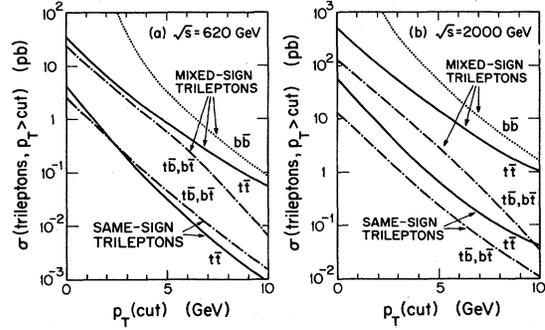
FIG. 3. Inclusive trilepton cross sections versus  $p_T$  cut in  $p\bar{p}$  collisions: (a)  $\sqrt{s}=620$  GeV, (b)  $\sqrt{s}=2000$  GeV. The  $b\bar{b}$ ,  $t\bar{t}$ , and  $t\bar{b}$  ( $b\bar{t}$ ) contributions are shown separately for mixed-sign trileptons and same-sign trileptons, for a single-lepton flavor as defined in Eqs. (2) and (3).
