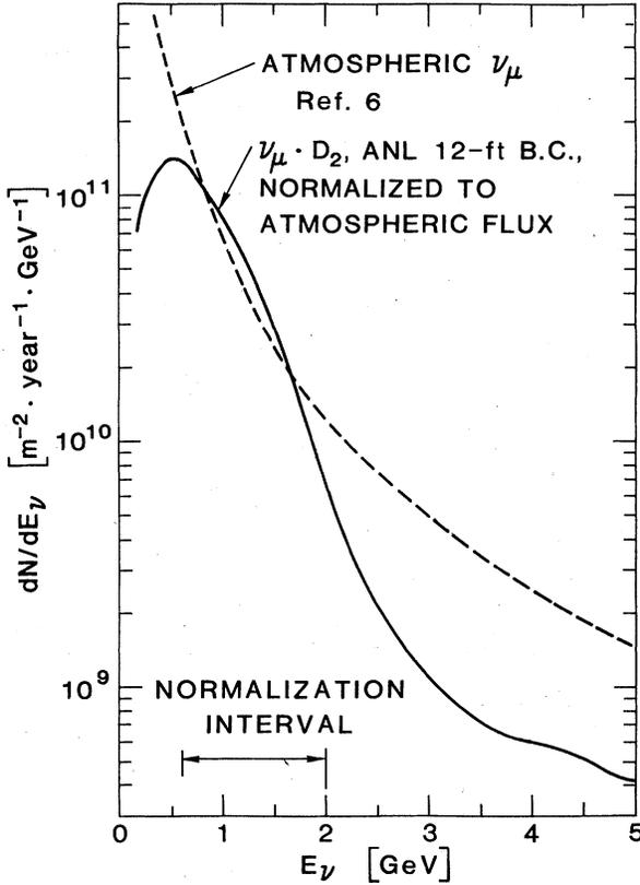
FIG. 1. Neutrino flux for our experiment (solid curve), normalized to the atmospheric  $\nu_\mu$  flux (dashed curve) in the interval  $0.6 \leq E_\nu \leq 2.0$  GeV.
