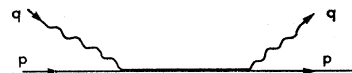
Fig. 1. s -channel Born approximation used as the "hard" part of the Compton amplitude.
