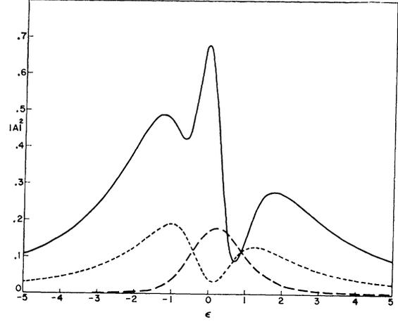
FIG. 3. Absolute squares of amplitudes for  $\gamma_{12}=0.75$ ,  $\gamma_{13}=0.55$ ,  $\gamma_{23}=0.75$ ,  $\phi=\frac{1}{6}\pi$ ,  $\theta=0$ , and  $\psi=0$ . The phase shifts for these amplitudes are shown in Fig. 4. The solid line is  $|A_{22}|^2$ , the short-dashed line is  $|A_{12}|^2$ , and the long-dashed curve is  $|A_{13}|^2$ .
