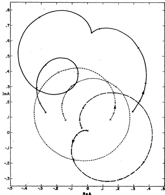
FIG. 4. Argand diagram for tripole with parameters listed in Fig. 3. The arrow denotes increasing energy. The curve begins at  $\epsilon = -5$ , and each cross bar signifies an increase of one unit of  $\epsilon$ . Again, the solid line is the Argand diagram for  $A_{22}$ , the short-dashed line is  $A_{12}$ , and the long-dashed curve is  $A_{13}$ .
