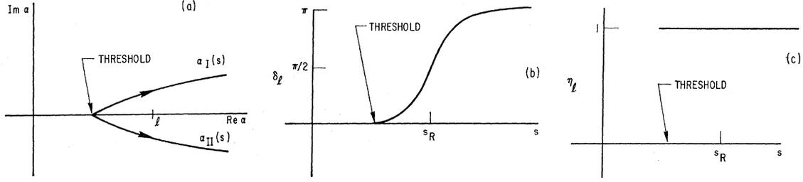
FIG. 1. (a) Pole and zero trajectories in the complex plane for the case of a completely elastic resonance. (b) Phase shift as a function of energy for the pole and zero trajectories in (a). (c) Elasticity as a function of energy for the pole and zero trajectories in (a).
