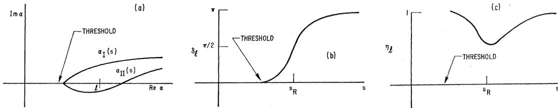
FIG. 2. (a) Pole and zero trajectories in the complex plane for the case of a slightly inelastic resonance. (b) Phase shift as a function of energy for the pole and zero trajectories in (a). (c) Elasticity as a function of energy for the pole and zero trajectories in (a).
