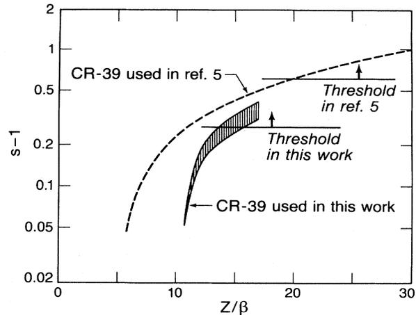
FIG. 1. Responses and detection thresholds for CR-39 detectors used in Ref. 5 and in this work. Although the CR-39 used in this work was less sensitive than that in Ref. 5, by etching for a longer time we were able to detect particles with  $Z/\beta$  lower than possible in Ref. 5.
