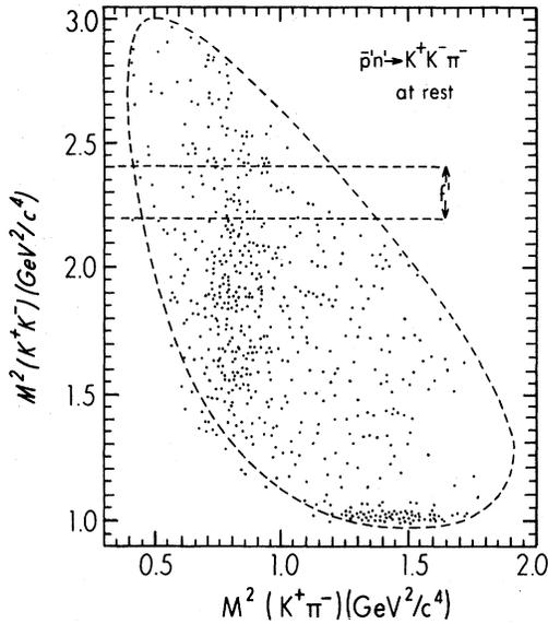
FIG. 3. Dalitz plot of the  $K^+K^-\pi^-$  events collected from annihilations at rest in deuterium. The boundary has been calculated assuming zero proton recoil momentum. The band over which the  $f'$  should be expected is indicated. Copious  $\phi$  and  $K^{*0}$  production is present but no evidence of  $f'$ . Upper limit of  $f'$  production is much less than the  $\phi(\rightarrow K^+K^-)$  production which is  $(3.5 \pm 0.6) \times 10^{-4}$ .
