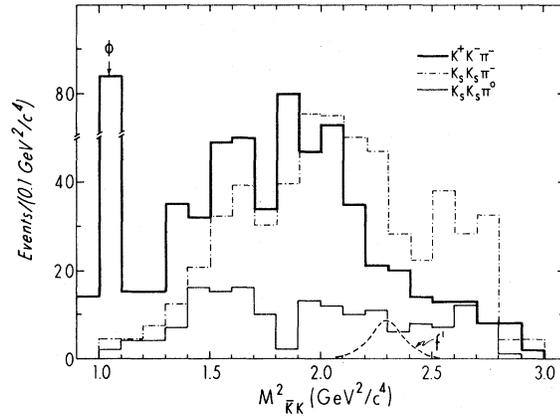
FIG. 5.  $\bar{K}K$  invariant-mass-squared distributions from Figs. 3 and 4 and Ref. 6 produced in  $\bar{p}N \rightarrow \pi K\bar{K}$  at-rest annihilations. The  $f'$  "signal" (arbitrary normalization) is indicated. No evidence of  $f'$  production is present in any of these channels.
