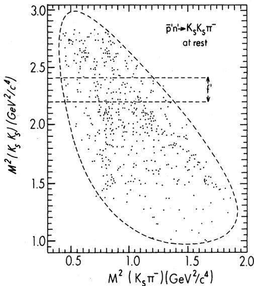
FIG. 4. Dalitz plot of the  $K_S K_S \pi^-$  events (two points/event) collected from  $\bar{p}d$  annihilations at rest. The boundary has been calculated assuming zero proton recoil momentum. The band over which the  $f'$  should be expected is indicated. Copious  $K^{*-}$  production is present but no evidence of  $f'$ .
