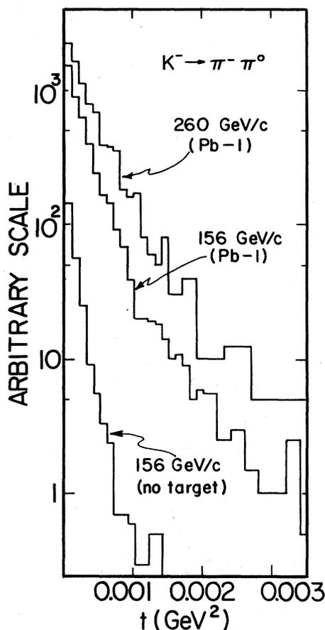
FIG. 11.  $t$ -distributions for  $K^- \rightarrow \pi^- \pi^0$  events accumulated with a lead target at 156 and 260 GeV/c, and no target in place at 156 GeV/c.
