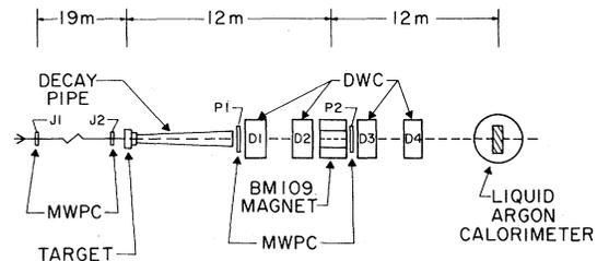
FIG. 2. Schematic diagram of the spectrometer.
