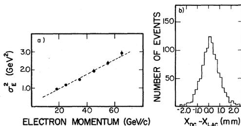
FIG. 4. Studies of the response of the LAC to bremsstrahlung electrons. (a) Energy resolution of the LAC (standard deviation squared) as a function of electron momentum. The dashed line corresponds to a resolution function of the form  $\sigma_E^2 = 0.18 + (0.20)^2 E$ , where  $E$  and  $\sigma_E$  are in GeV. (b) Plot of the difference between the  $X$  position of the electron as measured by the drift chambers and as measured by the LAC.
