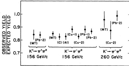
FIG. 12. Plot of the measured yield divided by expected yield for  $K^- \rightarrow \pi^- \pi^0$  events for different targets and both incident energies. (Points for which no target was present are indicated by the symbol MT.)
