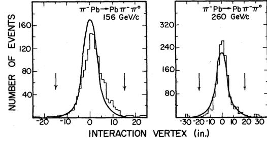
FIG. 14. Interaction-vertex distributions for the process  $\pi^- Pb \rightarrow Pb \pi^- \pi^0$  at 156 and 260 GeV/c. The smooth curves are predictions of the Monte Carlo model normalized to the total number of events in the distributions. The limits indicated by the arrows were used to define interactions in the target.
