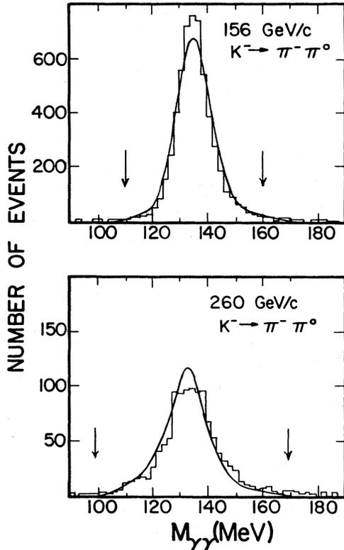
FIG. 6. Distributions of two-photon masses for  $K^-$ -decay events at 156 and 260 GeV/c. The arrows indicate the limits used to define  $\pi^0$ 's. The smooth curves are predictions of the Monte Carlo model normalized to the total number of events in the distributions.
