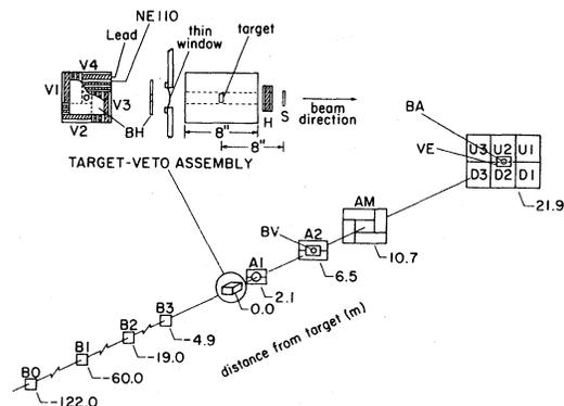
FIG. 5. Schematic of the arrangement of scintillation counters used in the trigger.
