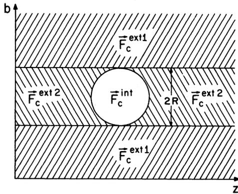
FIG. 20. Definition of the regions over which the electromagnetic form factor is calculated.
