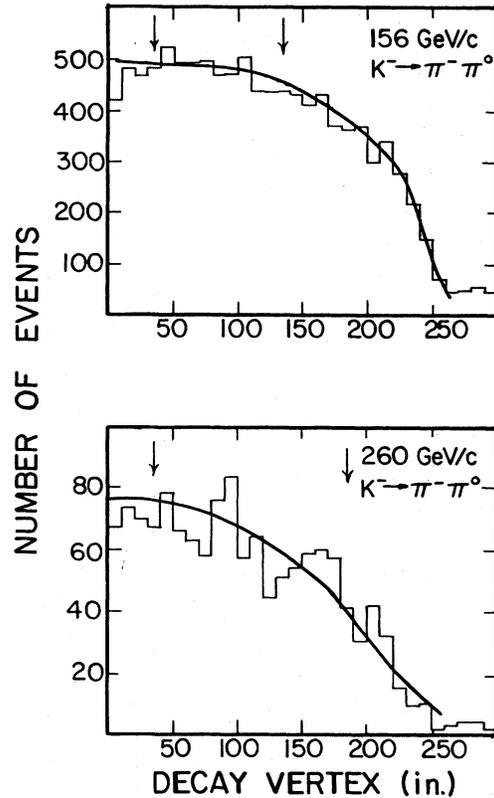
FIG. 7. Decay-vertex for  $K^- \rightarrow \pi^- \pi^0$  events at 156 and 260 GeV/c. The arrows indicate the data sample chosen for studies of resolution and normalization. The smooth curves are predictions of the Monte Carlo model normalized to the number of events between the arrows.
