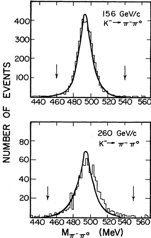
FIG. 8. Distributions in the  $\pi^-\pi^0$  mass for  $K^-\rightarrow\pi^-\pi^0$  decays at 156 and 260 GeV/c. The smooth curves are predictions of the Monte Carlo model normalized to the total number of events in the distributions. The arrows indicate the limits used to define the  $K^-\rightarrow\pi^-\pi^0$  signal.
