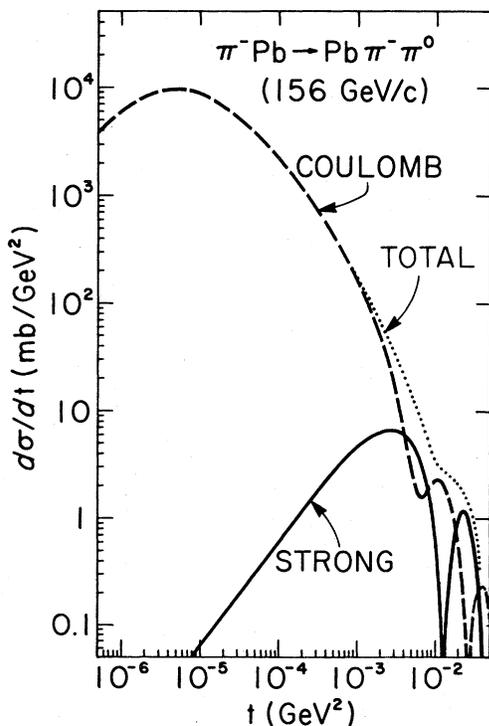
FIG. 21. Relative contributions from the Coulomb, the strong terms, and total cross section in coherent  $\rho^-$  production at 156 GeV/c on lead (Pb-2 in Table VI), prior to the introduction of resolution smearing.
