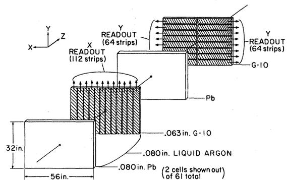
FIG. 3. Schematic diagram for the assembly of the liquid-argon calorimeter.
