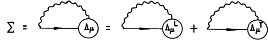
FIG. 1. Diagrammatic representation of the self-energy kernel \Sigma of the linear Schwinger-Dyson equation, in terms of the longitudinal and transverse vertex functions.
