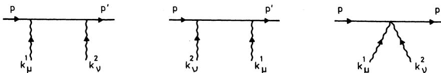
FIG. 11. Matter interacting with two photons at lowest order.
