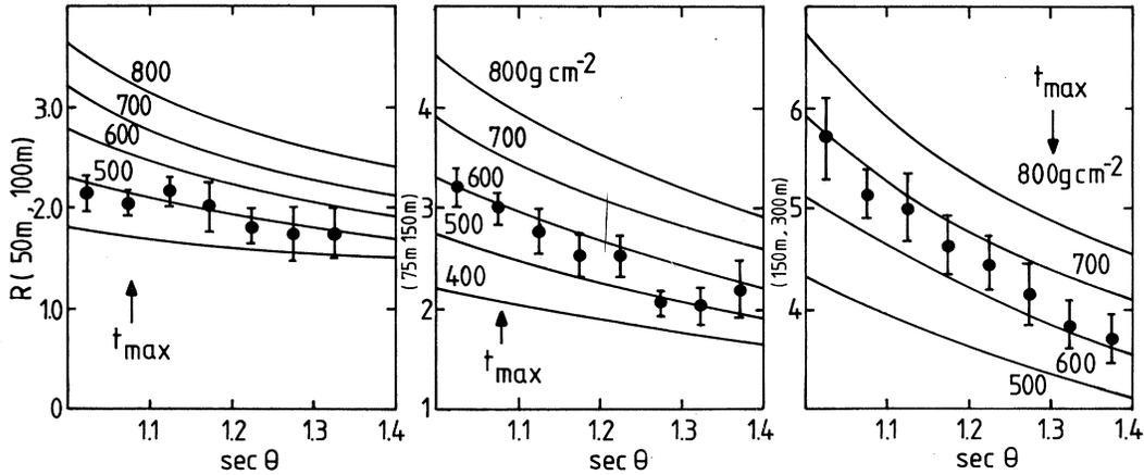
FIG. 2. The measured variation of the density ratio  $R(r_1, r_2)$  with zenith angle for showers with primary energies of  $6.5 \times 10^{15}$ ,  $2.3 \times 10^{16}$ , and  $2.0 \times 10^{17}$  eV recorded with the three sizes of Cherenkov-light array. Also shown (solid lines) are our computer simulations of these ratios for showers with the indicated depths of electron cascade maximum.
