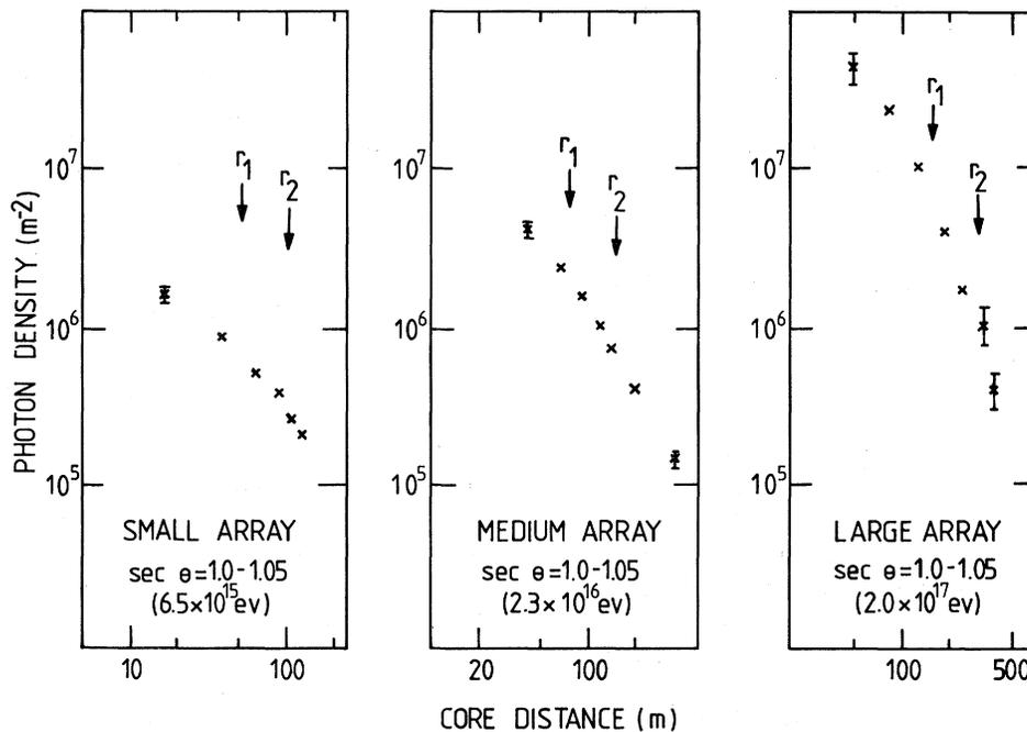
FIG. 1. The measured optical Cherenkov lateral distribution functions for EAS of energies  $6.5 \times 10^{15}$ ,  $2.3 \times 10^{16}$ , and  $2.0 \times 10^{17}$  eV. The measurements were made using arrays of three sizes. The distances  $r_1$  and  $r_2$  at which the density ratio  $R(r_1, r_2)$  is defined are shown for each array.
