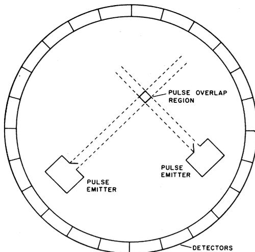
FIG. 1. Space-time event coordinate-measuring device. Two light pulses are emitted so that they overlap at the point in space and at the time where a charged particle is to be detected. If the particle absorbs a photon from each pulse, it can emit a photon that can activate one of the detectors surrounding the overlap region.
