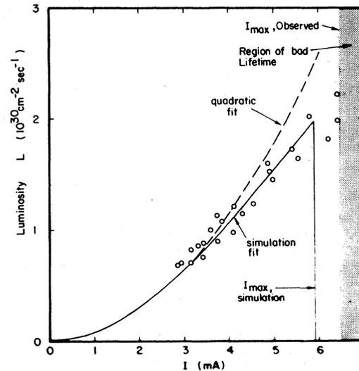
FIG. 2. Dependence of luminosity on current. Comparison between experiment and theory at CESR. Limits imposed by bad beam lifetime are shown. For these data the tune parameters were 9.415 for  $\nu_{x0}$  and 9.345 for  $\nu_{y0}$ .
