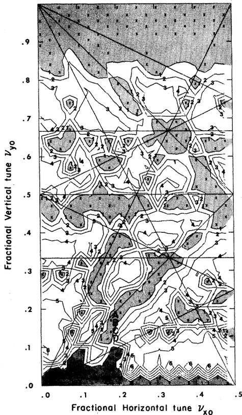
FIG. 1. The tune plane as studied analytically [the straight lines indicate instability thresholds of (1)] and numerically (the contours are curves of constant relative luminosity, very roughly in units of  $10^{30} \text{ cm}^{-2} \text{ sec}^{-1}$  for typical parameters). The crosses indicate bad lifetime and the shaded regions have very low luminosity. Points labeled *A*, *B*, *C*, and *D* identify lattice points for an investigation described in the text.
