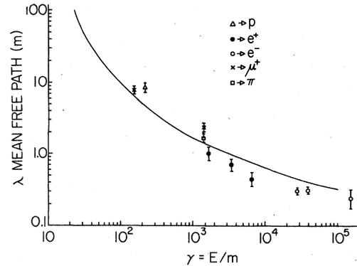
FIG. 2. Electron-pair mean free paths in nuclear emulsions as a function of  $\gamma$  ( $\approx E/M$ ) for electrons (Refs. 3, 15-20), protons (Ref. 6), muons (Ref. 7), and pion (this experiment). The theoretical curve is given by Eq. (5) of Ref. 3.
