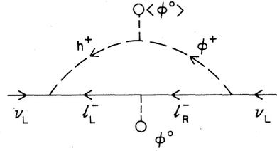
FIG. 3. Finite and calculable one-loop contribution to  $\bar{\nu}_L(\nu_L)^c$  in the model with singly charged singlet scalar  $h$ .
