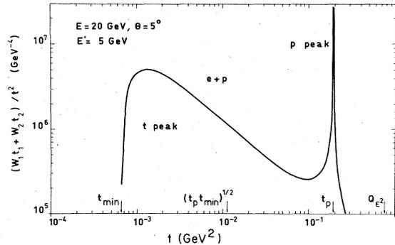
FIG. 4. Differential hard bremsstrahlung cross section versus the squared momentum transfer emphasizing the importance of  $t$  peak for very inelastic scattering. The small- $p'$  peak is not shown.
