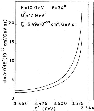
FIG. 3.  $e$ - $p$  elastic-peak spectrum: comparison between the nonperturbative (lower curve) and the one-photon-emission (upper curve) cross section.
