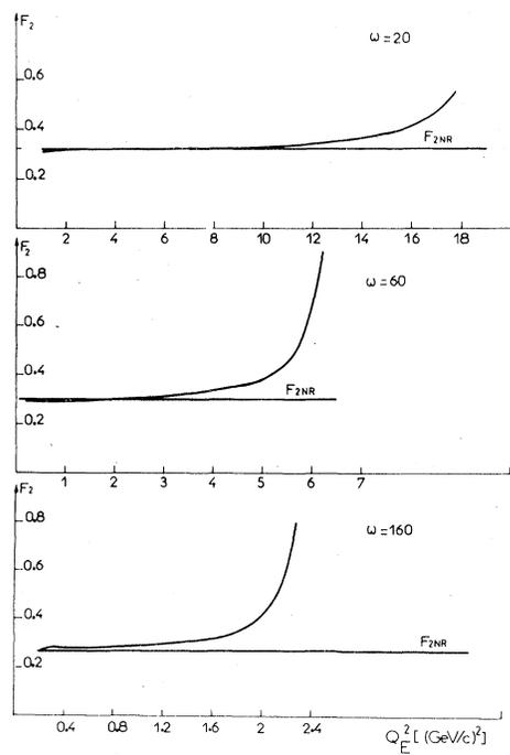
FIG. 6. Radiative corrections for  $\mu+p$  scattering at  $E=219$  GeV for various  $\omega$  values. The horizontal lines represent the Feynman scale-invariant, nonradiative structure function.
