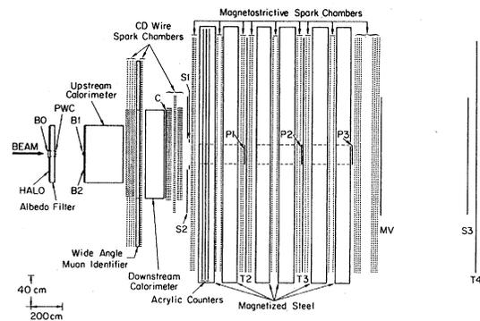
FIG. 1. Plan view of the experimental apparatus. A 400-GeV/c proton beam is incident from the left.  $B0$ – $B2$ ,  $H$  (halo),  $C$ ,  $S1$ – $3$ ,  $ACR1$ – $3$  (acrylic),  $T2$ – $4$ ,  $MV$ , and  $P1$ – $3$  are all counters used in trigger logic or event selection.
