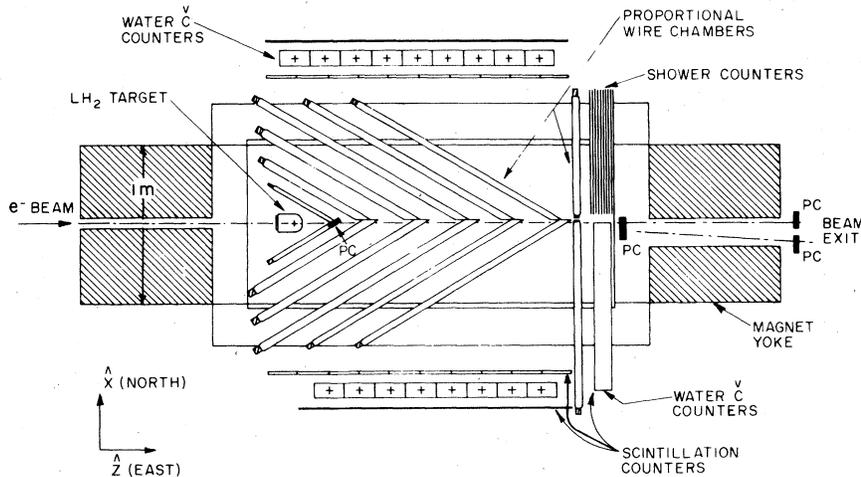
FIG. 1. Plan view of the apparatus.
